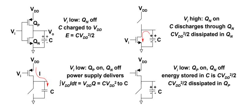
$CV_{DD}^{2}$  total power dissipated
