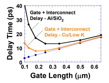
AI:  $\rho = 3 \mu\Omega$ -cm Cu:  $\rho = 1.7 \mu\Omega$ -cm SiO<sub>2</sub>:  $K_{ox} = 4$ Low K:  $K_{ox} = 2$ AI/Cu: 0.8 μm thick AI/Cu: 43 μm long
