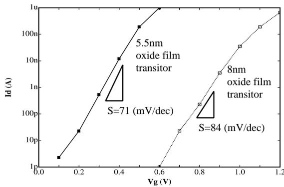
Fig.5 Vg-Id characteristic of the memory cell transistors
