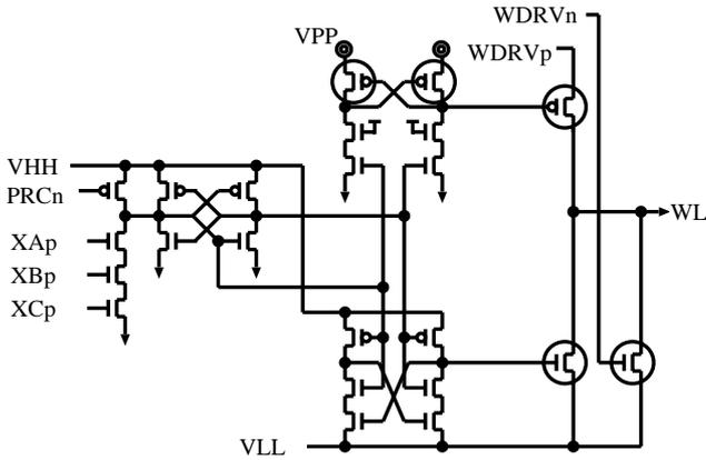
Fig.1 The row decoder circuits of the two macros
