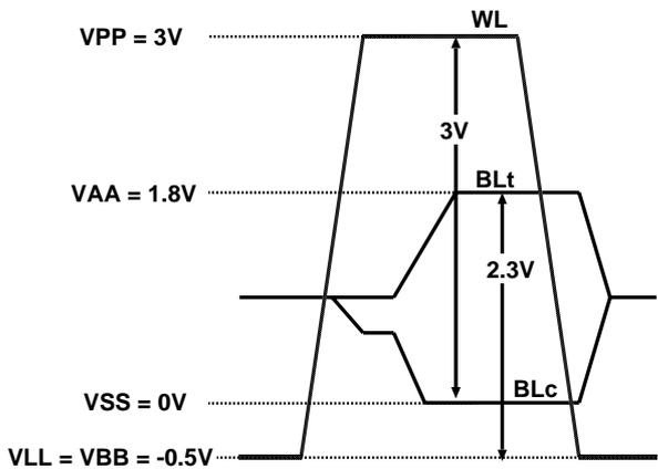
Fig.2 The waveform of the negative WL architecture
