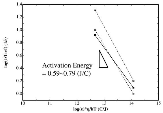
Fig.7 The temperature dependence of the retention time of the negative WL architecture
