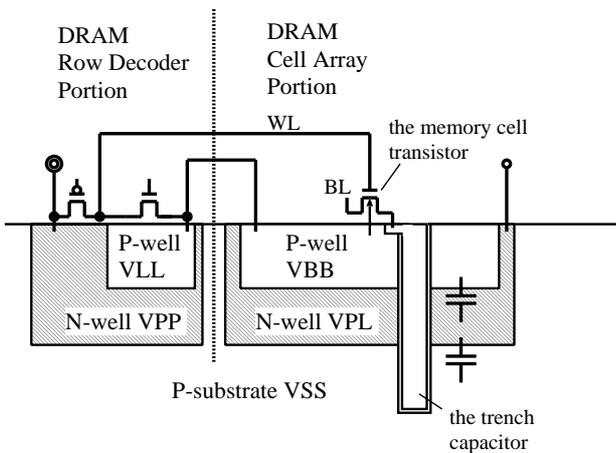
Fig.3 The cross section of the well structure for the negative WL architecture
