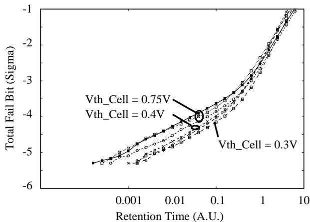
Fig.6 The retention characteristics of the negative WL architecture with the various Vth memory cell transistors
