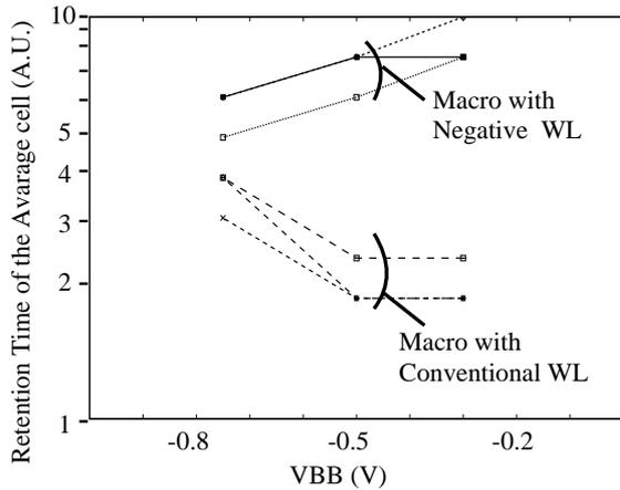
Fig.4 The retention time comparison between the negative WL architecture and the conventional WL architecture
